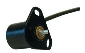
The output of a rotary hall sensor is a voltage which changes in direct proportion to the shaft angle. A constant voltage is required across the supply and ground wires of the sensor. No internal end stops are fitted, so continuous rotation is possible. The sensor consists of a Hall Effect element, a shaft and a magnet. When the angular position of the sensor changes relative to the magnet, the change In magnetic field in the sensor results in a change in output voltage.
